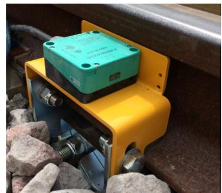
**Note: If required by site conditions the sensor can be reversed on the sensor mounting plate such that the cable exits in the opposite direction.**
