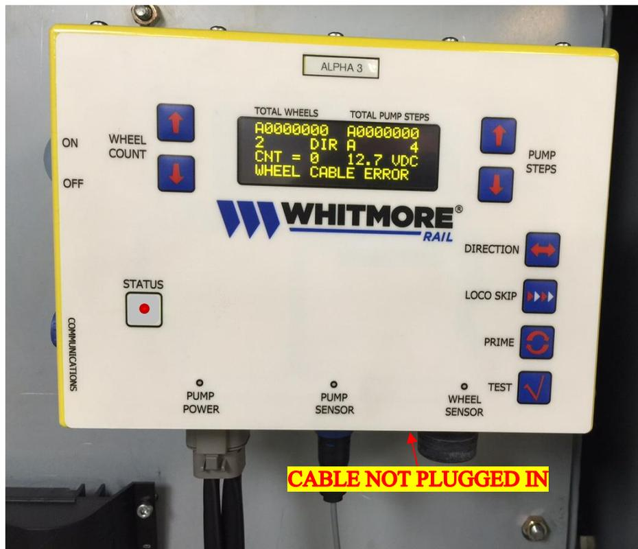
This error will only occur upon powering on the controller with the wheel sensor cable being unplugged or not having a good connection. The STATUS LIGHT (13) will illuminate red and the message WHEEL CABLE ERROR will display on line 4. To fix this power down the controller and ensure the wheel sensor cable is properly connected. You must power cycle the controller in order to clear the error. (**NOTE:** cables should never be connected/disconnected with the controller powered on)
